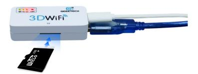
Step 4. Long press the hole labeled with "set" with a pin, until the Wi-Fi indicator light turns dim and flickers quickly. Loosen the pin and 3D Wi-Fi will enter the config mode. You could finish Wi-Fi configuration on EasyPrint 3D App.
