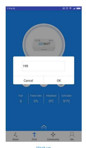
Step 2. Click [Heat up] button Heat up and you will see the extruder temp increases until it reaches the target one.
